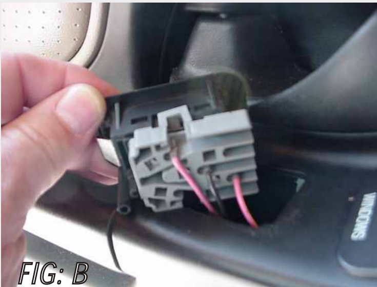
FIG. B: Below shows rear of OEM rocker switch.
